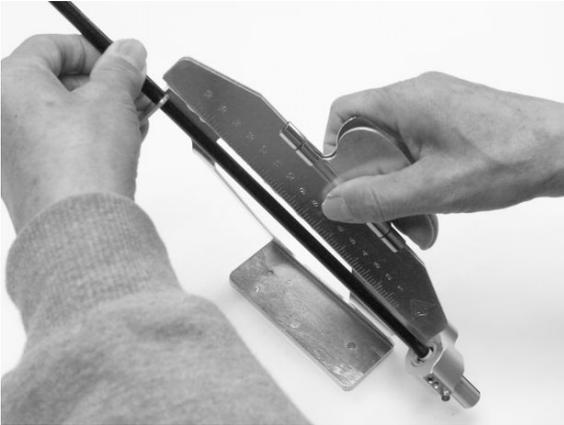
Put the clamp on the base by first attaching the clamp to the magnet. Then place the bottom end on the base. Finally, press the top end against the shaft.
