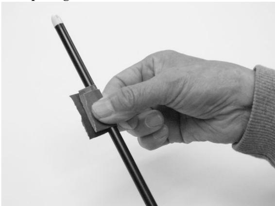
Rough the surface of the shaft a length of 9 inches below the nock with #800 sandpaper to ensure that the feathers are bonded firmly.
