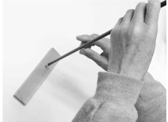
Strike the arrow down onto a piece of hard wood to set the point.
