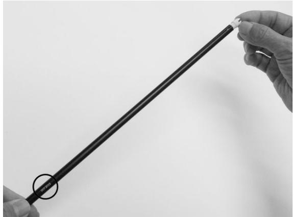
Push the nock in a little and turn it around fully to spread the bond evenly on the root of the nock. Align the groove of the nock with the XX75 mark.
