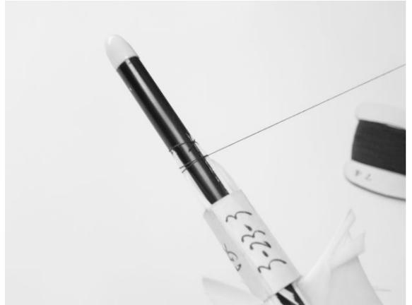
When the thread comes to 1mm above the hairline, wind 2 to 3 times as to press it down toward the nock.
