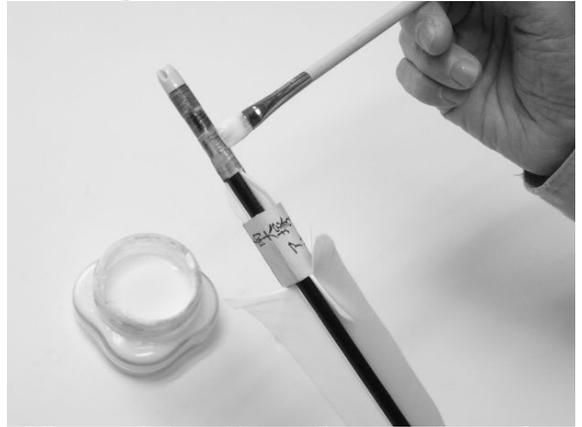
Dilute wood glue with a small amount of water. Coat the threads equally while rotating the shaft. Coat the space between the threads. Apply a second coat once the glue dries well.
