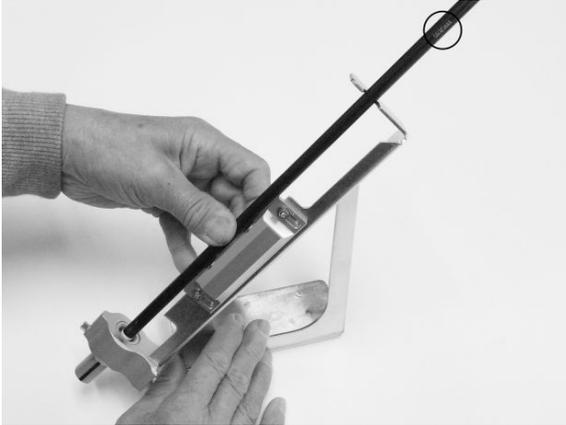
Insert the nock deeply in the nock supporter and placed so that the XX75 mark is aligned with the mark on the knob.
