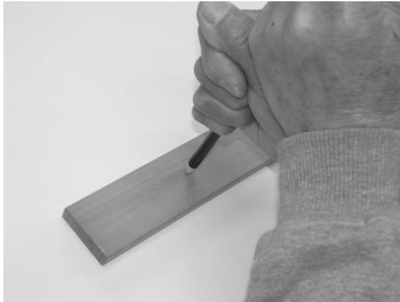
Once the position has been determined, press straight down onto a piece of hard wood to push in the nock.
