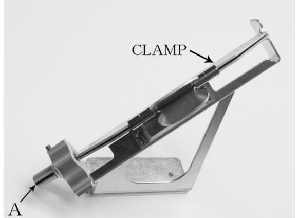
Make sure that a mark (A) on the knob is aligned with the clamp.
