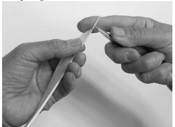
Hold the feather with the quill facing up. Place the knife blade on the back of the quill and use your index finger to press the quill against the blade and shave the soft part by sliding the knife to the end of the quill.
