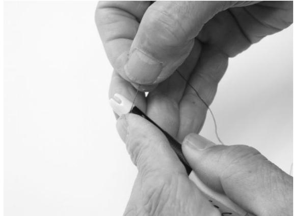
From the bottom of the nock wind the thread without leaving spaces.
